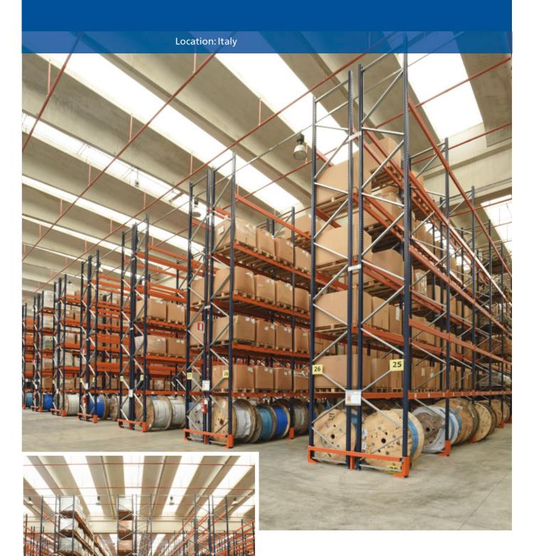
Trasgo's logistics centre in Italy is sectored into four different areas to organise the goods of Enel — an important customer who distributes electricity — according to product characteristics and to comply with local fire regulations. Mecalux supplied pallet racking that offers a storage capacity of more than 20,200 pallets and ensures optimal management of any product.
