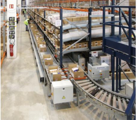
Mecalux automated a portion of the warehouse that AS Healthcare owns close to Paris in order to guarantee efficient picking, save on logistics costs and reduce the margin of errors during handling. The solution consisted of live pallet racking with the pick-to-light system and a conveyor circuit with rollers that joined the prep zone to the sorting and consolidation areas.
