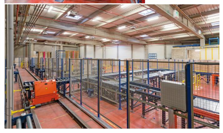
The conveyor circuit also incorporates a full pallet stacker, which can lift the pallets to place them on slave pallets, and a station where empty pallets are stacked and unstacked.
