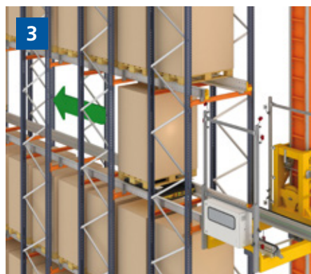
3. The automatic shuttle raises the load slightly and slots it into the storage channel. It slides with the pallet to the first open location and, once there, lowers the pallet, setting it on top of the rail.
