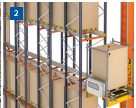
2. The stacker crane scoops up the pallet with several chains installed in the cradle and moves to the channel assigned by the WMS.
