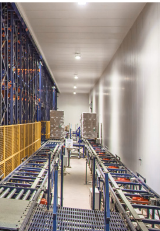
1. The Pallet Shuttle in the stacker crane's cradle waits for the pallet's arrival from the checkpoint.
