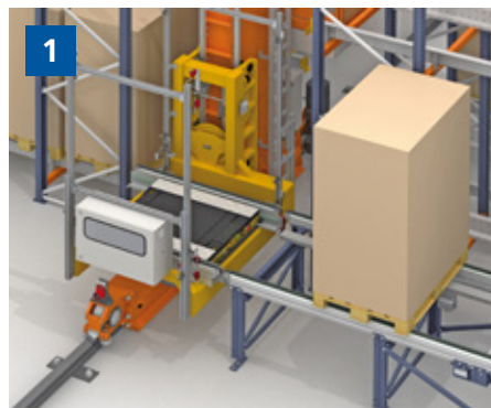
1. The Pallet Shuttle in the stacker crane's cradle waits for the pallet's arrival from the checkpoint.
