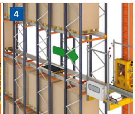
4. The stacker crane waits for the Pallet Shuttle to finish and move automatically back onto the cradle.
