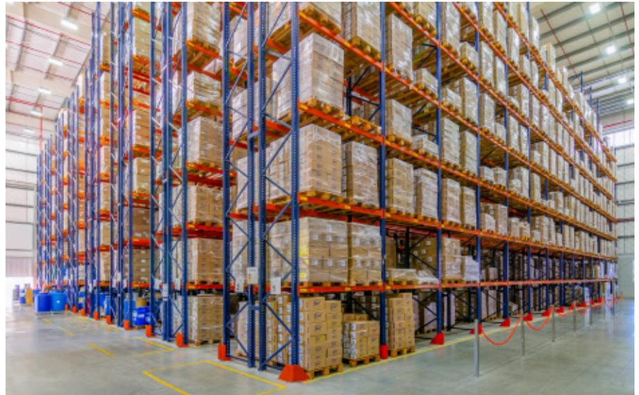
Pallets with raw materials are deposited in the lower levels of the racks because they are heavier and more accessible
