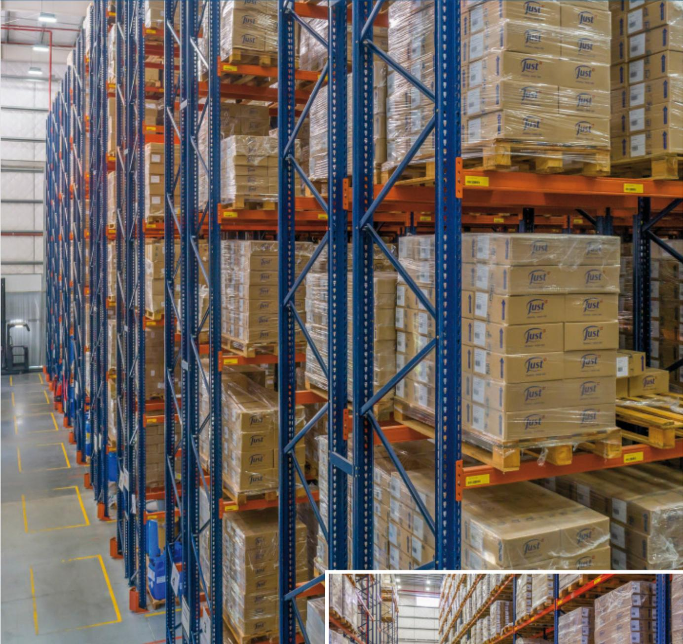
Just, a renowned cosmetics brand, has opened a new 1,681 m<sup>2</sup> warehouse in Buenos Aires (Argentina). Its operation consists of supplying production lines with raw materials and, at the same time, receiving finished products. Mecalux, to make the most of the centre, has equipped it with 14 m high pallet racks with a capacity for 3,800 pallets. The direct access facilitates the handling of goods.
