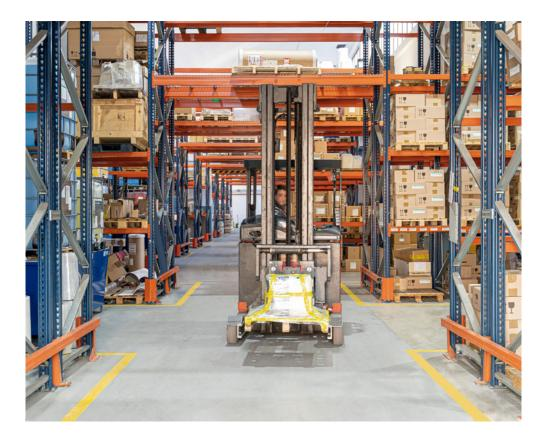
This versatile storage system is ideal for storing a large number of pallets of varying weights and volumes. At the same time, direct access to all products facilitates the handling of the goods and order preparation.
