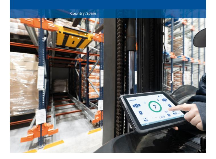
The warehouse of bakery goods and pastry producer Nicopan in Atarfe, Spain, is divided into multiple cold stores that Mecalux has equipped with the semi-automatic Pallet Shuttle system. In total, 9,931 pallets with finished products and raw materials are stored. Mecalux has also implemented the Easy WMS warehouse management system, as well as the Pallet Shuttle control software, prepared to direct the motorised shuttles used in this storage system.
