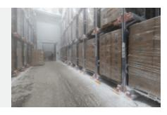
Taking this into account, Mecalux has fitted out the five cold stores with the semi-automatic Pallet Shuttle system. This high-density storage system uses an electric shuttle to load and unload pallets inside storage channels. It was chosen based on the following factors:
