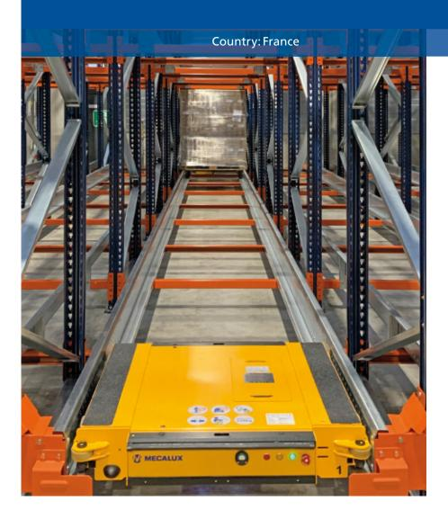
Sauce manufacturer Manna Foods has renovated its warehouse in Wijnegem, Belgium, with the installation of the Pallet Shuttle system from Mecalux. This solution makes the most of the available space to provide greater storage capacity: 1,120 pallets in just 350 m². The secret? A motorised shuttle tasked with handling the goods, thereby streamlining pallet entries and exits.
