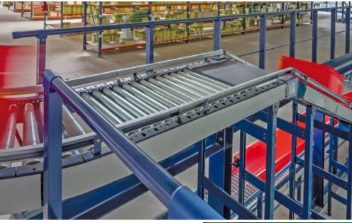
The conveyor belts allow height differences to be overcome and movements to be carried out at different levels, while the swing conveyors allow the passage of the operators
