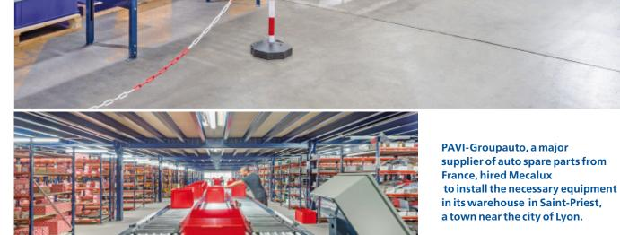
The supply included two levels of mezzanines, racking, conveyor belts and automatic sorters, as well as the Mecalux Easy WMS warehouse management system.
