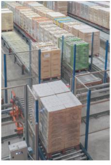
A shuttle is responsible for connecting the output stations with different order consolidation channels
