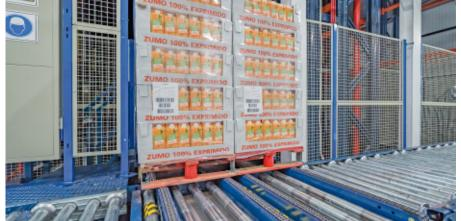
To store 800 x 1,200 mm sized pallets of indiscriminate depth with the utmost security, cross-ties were put in the racks, as shown in the picture below on the right.
