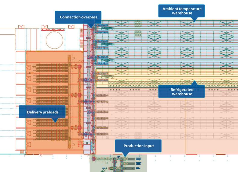
is for more than 23,000 pallets, 1,200 x 800 mm in size, 1,700 mm high and weighing 1,050 kg each. If all the pallets were 600 x 800 mm sized, the storage capacity would increase to more than 46,000 pallets
