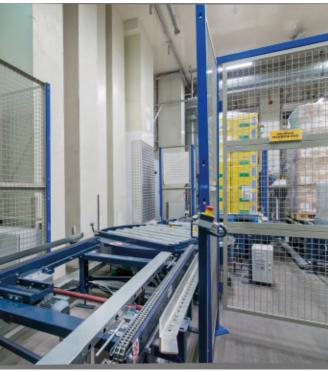
Mecalux has installed a conveyor tasked with moving goods directly from the NUTRICIA production centre to the warehouse's dispatch zone. This conveyor system cuts out the use of traditional handling equipment to shift goods between two points. By lessening manual load handling, this increments general safety in the installation significantly.
