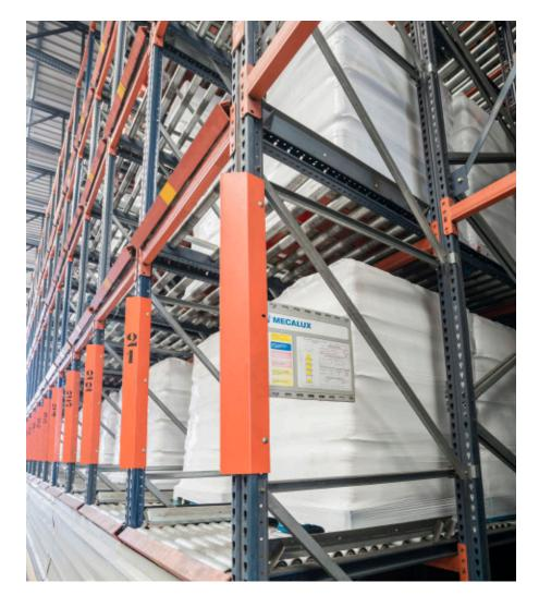
The live racking ensures perfect rotation of the goods, by applying the FIFO criterion (first in, first out), i.e., the first pallet to enter is the first to leave.
