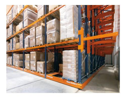
Movirack mobile pallet racks are particularly suitable for frozen-storage installations such as Sabarot's, as they reduce energy consumption thanks to the optimum distribution of cold between the pallets
