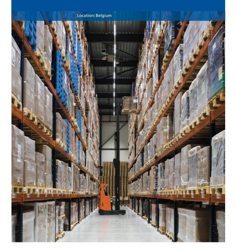
The logistics operator Van Rooijen has furnished its new warehouse in Turnhout (Belgium) with pallet racks from Mecalux that can hold a total of 32,500 pallets. Besides providing the optimal storage capacity to house all its customers' products, this system facilitates direct access to the merchandise, thus speeding up storage and order processing tasks.
