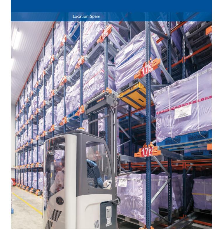
In recent years, the meat company called El Encinar de Humienta has made an extensive investment aimed at improving its infrastructures and processes. For this reason, it has opened a new 1,000 m² freezer space that Mecalux has equipped with the semi-automatic Pallet Shuttle system. There it deposits 1,997 pallets with finished products, ready to be distributed to its customers in Spain, Europe and Asia.
