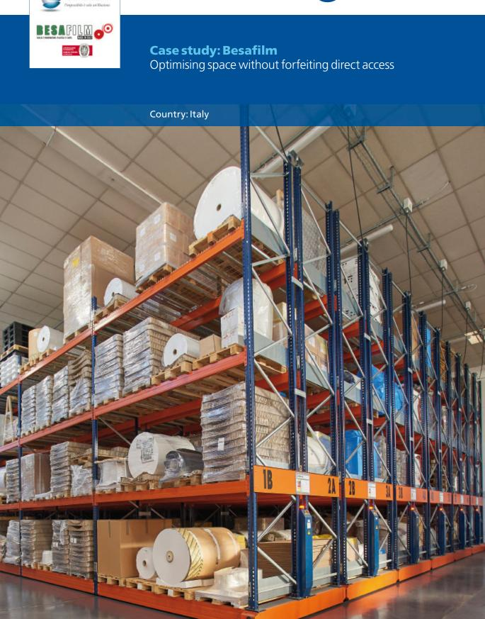
Besafilm has equipped its warehouse in Colognola ai Colli, Italy, with Movirack mobile pallet racking by Mecalux. This high-density system leverages all available space to provide storage capacity for 2,032 pallets. At the same time, it offers direct access to goods the moment a working aisle is opened.
